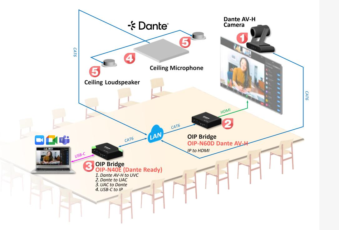
OIP-N40E (Dante Ready) combines with the OIP-N60D Dante AV-H to connect Dante audio and video devices in the conference room, while also linking to in room displays.
